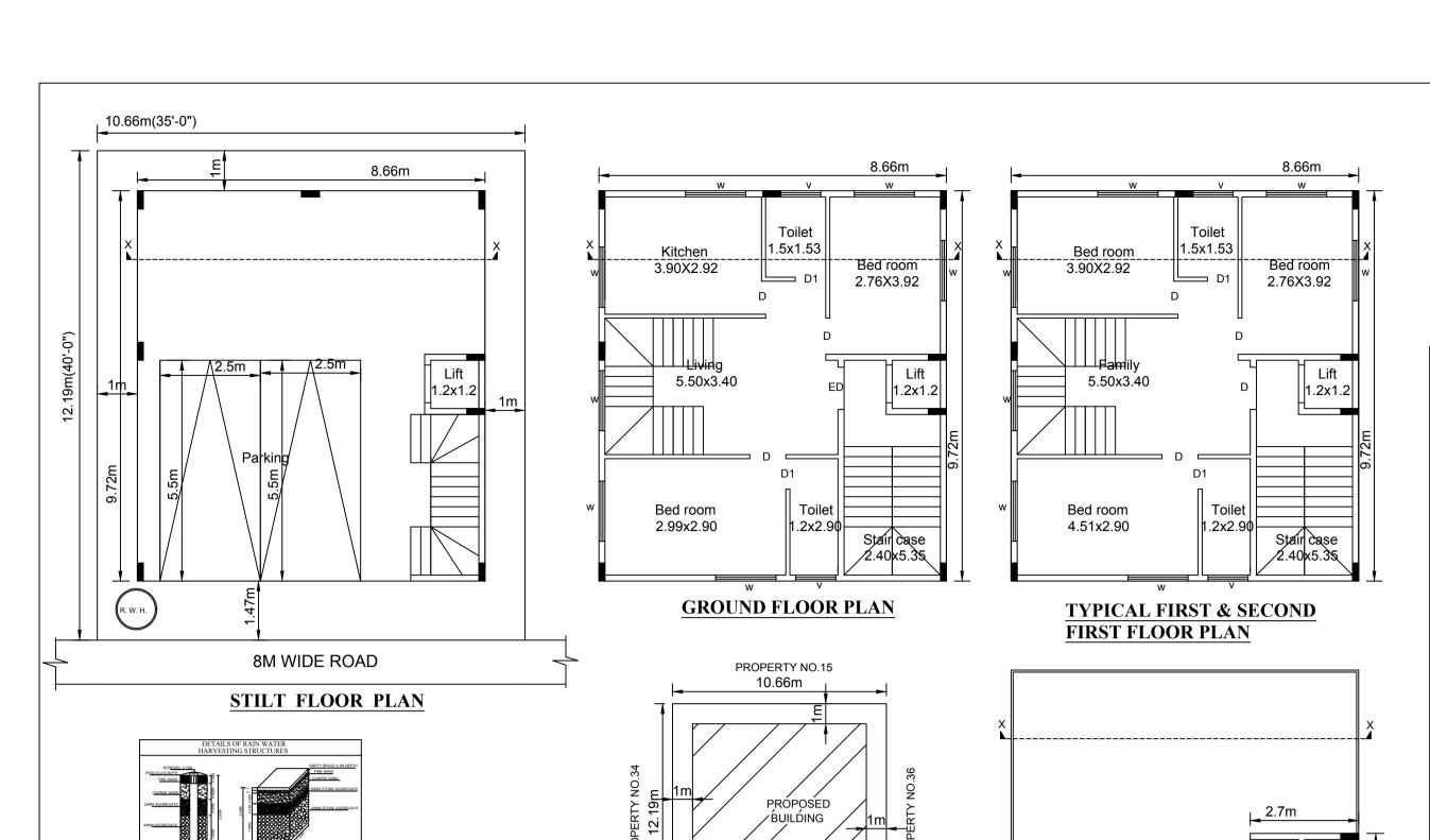
8M WIDE ROAD SITE PLAN SCALE(1:200) —HEAD ROOM —PARAPET WALL —R C C ROOF ----0.15 TH WALL RCCROOF —0.15 TH WALL
